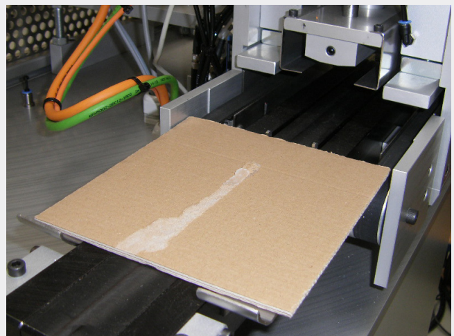
Ejection of the lower cardboard for visual examination.
