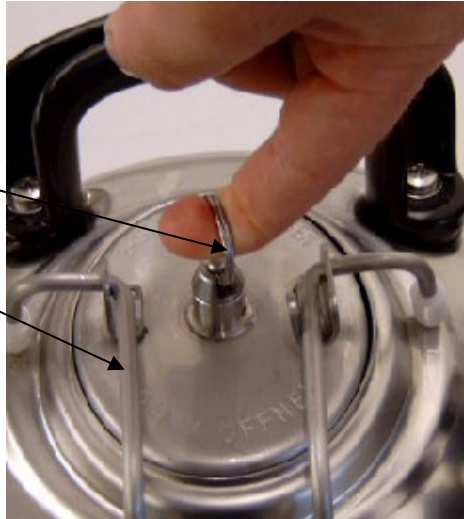
Picture: Pressure vessel, safety valve
