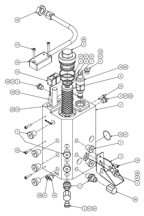
Illustration: Single Stream Filter Manifold Assembly, SR5/10
