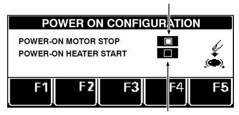
This parameter may not be programmed until it is activated. To activate, turn the Input Wheel.
