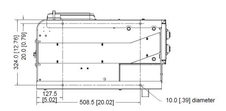
Installation & Clearance Dimensions: DM SR5: 5 kg (10 lb) Hopper Capacity
