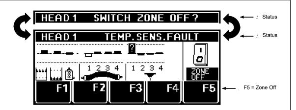
Advance to the temperature zones display to see which zone is affected. The two status lines shown above will alternate in this mode. As seen above, the question mark is placed on the zone with the faulty sensor (i.e., Head #1). After troubleshooting the fault (reference the Error Indication Alarm Troubleshooting Guide on the previous pages of this chapter) and solving the problem with the sensor, press the RETURN button.
