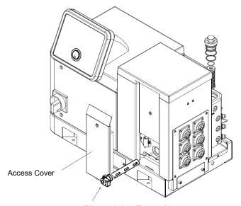
Filter and shutoff assembly: Turn knob to left position = closed/ OFF Turn knob to right position = open/ ON (shown)
