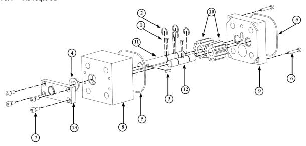
10.8.3.5 Single Gear Pump Assembly 20 cc/rev., PN 109694
