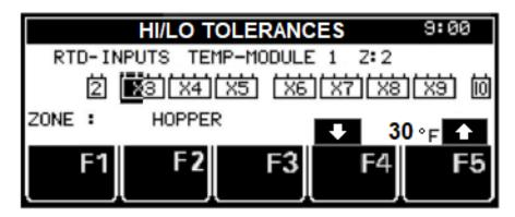
On this screen, use the Input Wheel to select the zone and buttons F4/F5 to change the tolerance for the selected zone. Picture above shows the hopper zone is selected and the tolerance is +/-30°F. It is not necessary to confirm with the Enter Knob. After all zones have been programmed, leave this screen by pressing the Return button.
