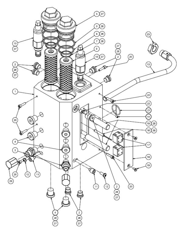
Illustration: Dual Stream Filter Manifold Assembly, SR5/10
