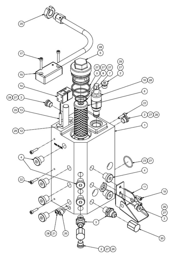
Illustration: Single Stream Filter Manifold Assembly, SR5/10
