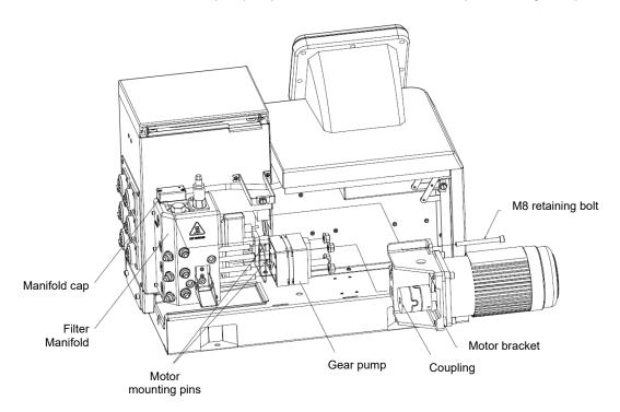
Gear Pump Model with Single Stream Manifold, shown from the rear
