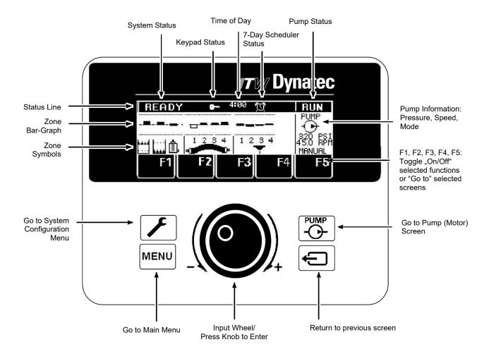
The Overview Screen gives a comprehensive view of the status of each of the temperature zones and the system as a whole. It gives the status, mode and speed of the pump.
