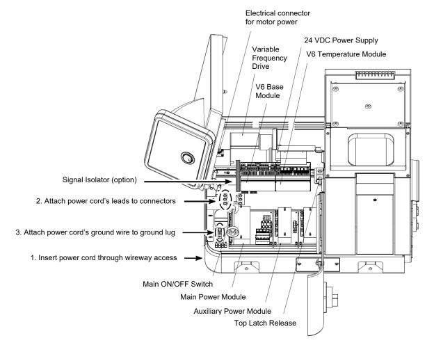
Main Power Installation & Internal Components
