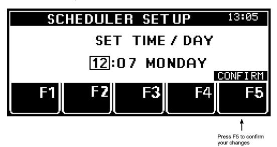
Turn the Input Wheel to select the item to be changed. Press the Enter Knob. Turn the Input Wheel to the desired time/ day and press F5 to confirm your entry.
