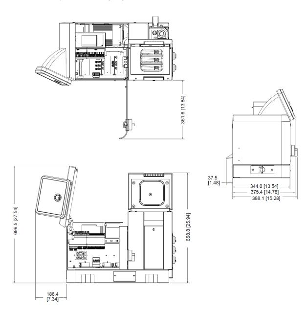
Installation & Clearance Dimensions: DM SR5: 5 kg (10 lb) Hopper Capacity
