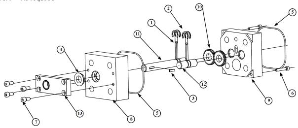
10.8.3.7 Dual Gear Pump Assembly 0.55 cc/rev., PN 109909
