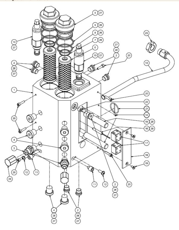
Illustration: Dual Stream Filter Manifold Assembly, SR5/10
