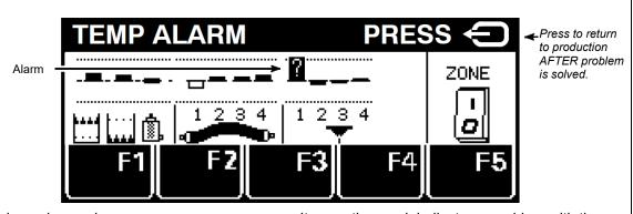
The alarm shown above can occur on any screen. Its question mark indicates a problem with the RTD sensor in the Head #1 zone.
