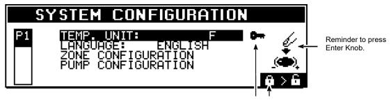
Selected parameter is locked and cannot be programmed without the access code.
