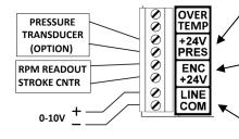
If the ASU is equipped with a digital pressure read-out, it connects to this terminal. The transducer type is two-wire 4-20mA.
