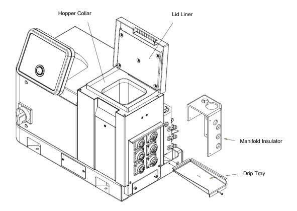
The unit is equipped with a removable stainless-steel drip tray under the filter manifold. Adhesive leaking from a gear pump's shaft seal will collect on the drip tray. The drip tray should be inspected monthly for adhesive residue. residue indicates that the pump seal is worn and needs to be replaced. See instructions in Chapter 8 for replacement of this seal.
