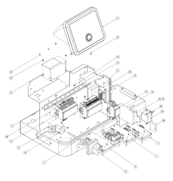
10.8.1.2 Hopper (Tank) Assembly, SR5/10
