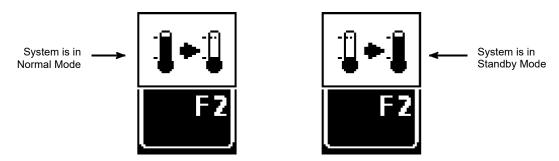
Press the Main Menu button, then press F2 to toggle between Normal mode (setpoints and pump are active) and Standby mode (setpoints are lowered and pump is stopped.) Confirm Standby mode by pressing F2 again. After making a change, a screen message will indicate, "Standby ON" or "Standby Off".
