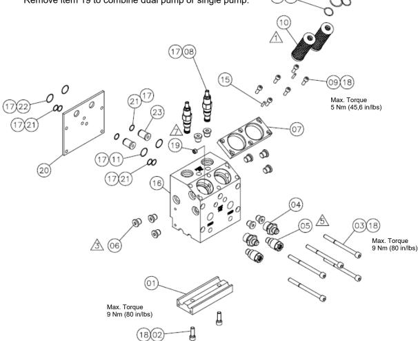
Illustration: Filter Manifold Assembly, Easy-Spin, for dual pump, PN 814016
