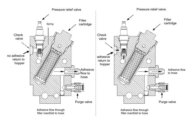
Operation of the Adjustable Adhesive Pressure Relief Valve
