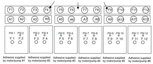
Up to six Filter manifolds with up to 24 Adhesive Ports
