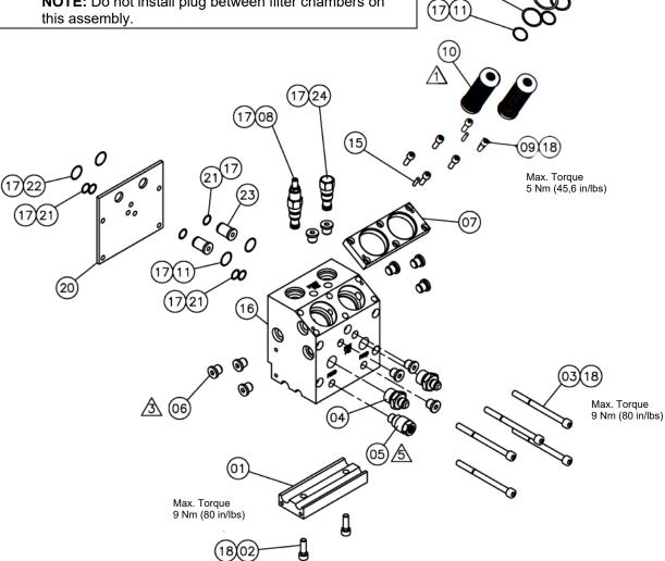
Illustration: Filter Manifold Assembly, Easy-Spin, for single pump, PN 825653
