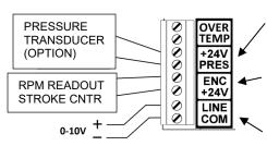
If the Melter is equipped with a digital pressure read-out, it connects to this terminal. The transducer type is two-wire 4-20mA.
