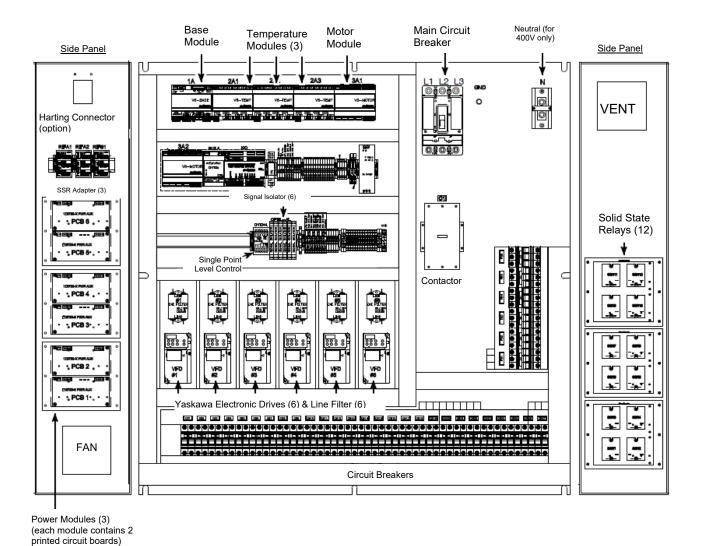
Typical Panel Box Layout with Options (Single Hopper model shown)
