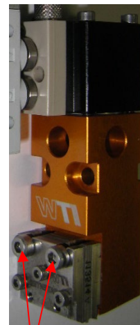
UFD High-Speed Nozzle's two mounting screws
