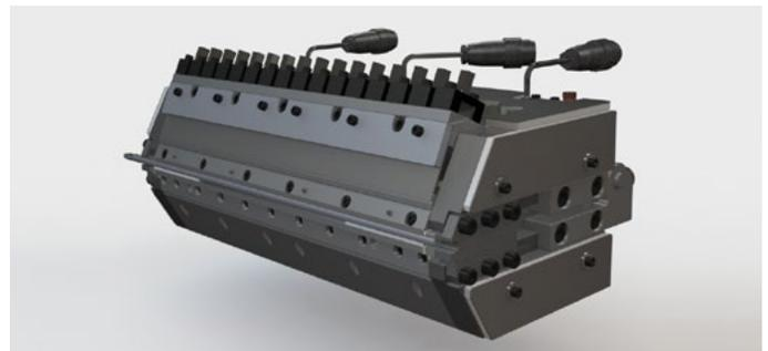
Rotary Rod with Flex Lip Slot Die
